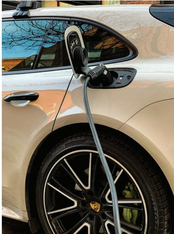
*On the electrical side, there is a 14 kWh lithium-ion battery with Porsche charging equipment. You can also recharge it on most public charges.*
